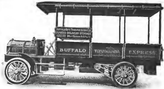
Three-ton, Four-cylinder, 40-h.p. Truck.
